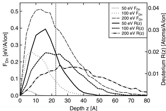
Fig. 4. SRIM analysis of the depth distribution of deposited energy from bombarding deuterium ions ( $F_{Dn}$ ) (thin lines) and the range of the ions  $R(z)$  (thick lines). The vertical line shows the size of the MD simulation box.
