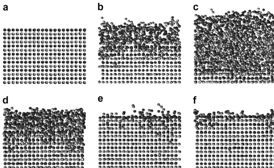
Fig. 3. Snapshots of (a) the initial WC lattice and after cumulative deuterium bombardment at (b) 50 eV, (c) 100 eV, (d) 200 eV, (e) 1000 eV and (f) 2000 eV. The lighter spheres represent C atoms and the darker ones W atoms.
