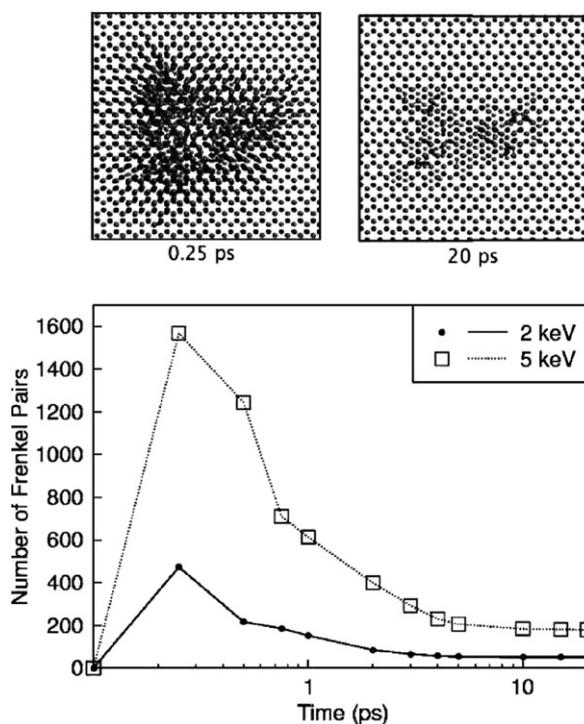
Fig. 1. Frenkel pair production as a function of time in 2 keV and 5 keV W-recoil cascades in WC. The figure also shows snapshots, taken at 0.25 ps (left) and at 20 ps (right), of a 5 keV cascade, where it can be visually seen that most of the damage recombines. The lighter spheres represent C atoms and the darker ones W atoms.
