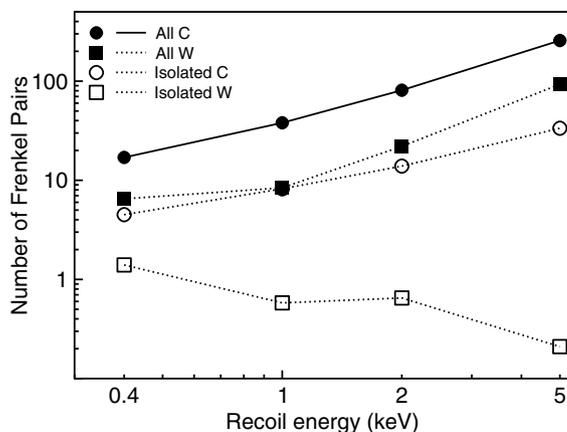
Fig. 2. Total and isolated defects after 0.4 keV, 1 keV, 2 keV and 5 keV W-recoil cascades. The isolated Frenkel pairs are not part of a defect cluster.
