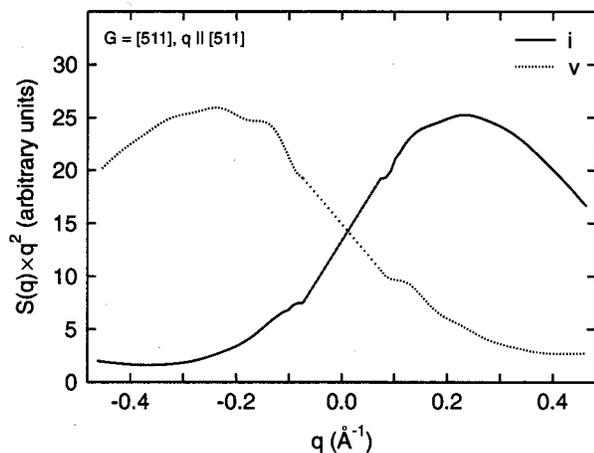
FIG. 3. Diffuse scattering of a vacancy (v) and  $\langle 110 \rangle$  dumbbell interstitial (i) in Si. The scattering is plotted in units of  $Sq^2$  vs  $q$ , where  $S$  is the scattering intensity and  $q$  the distance in reciprocal space to the Bragg peak  $G$ . The Bragg peak is left out of the figure, and the scattering lineshape of both defects interpolated in the middle to guide the eye.
