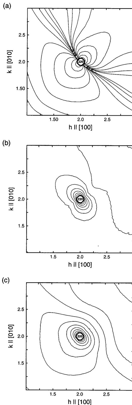
FIG. 4. Diffuse scattering iso-intensity curves around the (220) Bragg peak for three different vacancy structures in Ge. (a) shows the scattering for a vacancy with tetrahedral ( $T_d$ ) symmetry, i.e., all four atoms surrounding the vacancy relaxing inwards toward it; (b) shows one with  $D_{2d}$  symmetry, i.e., two bonded atom pairs forming symmetrically on both sides of the vacancy; and (c) shows a lower-symmetry structure characteristic of negatively charged vacancies.
