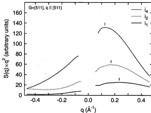
FIG. 6. Simulated diffuse scattering for three interstitials clusters  $i_j$  in Si, where  $j$  denotes the number of extra atoms in the cluster. The Bragg peak has been left out of the figure. The locations of the maxima on the positive side are indicated by tiny vertical lines. The relaxation volumes of the mono-, di- and tetrainterstitial used here are  $+1.5$ ,  $+2.6$  and  $+4.3$  atomic volumes, respectively.
