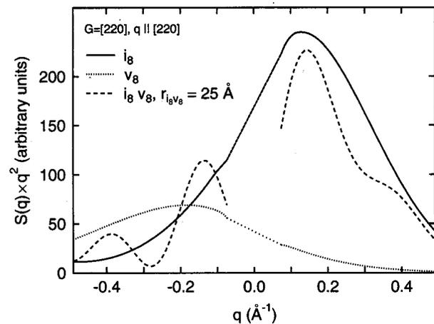
FIG. 9. Diffuse scattering of an octa-vacancy ( $v_8$ ) and octa-interstitial ( $i_8$ ) in Si, and a defect consisting of both the  $v_8$  and  $i_8$  separated by 25 Å. The Bragg peak is left out of the figure, and the scattering lineshape of the single clusters interpolated in the middle to guide the eye. The relaxation volumes of the  $i_8$ ,  $v_8$  and combined  $i_8 v_8$  defects used here are +8.0, -4.0 and +4.0 atomic volumes, respectively.
