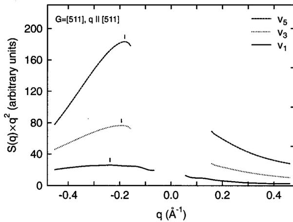
FIG. 5. Simulated diffuse scattering for three vacancy clusters  $v_j$  in Si, where  $j$  denotes the number of vacancies in the cluster. The Bragg peak has been left out of the figure. The locations of the maxima on the negative side are indicated by tiny vertical lines. The relaxation volumes of the mono-, tri- and pentavacancy used here are  $-1.5$ ,  $-3.2$  and  $-5.3$  atomic volumes, respectively.
