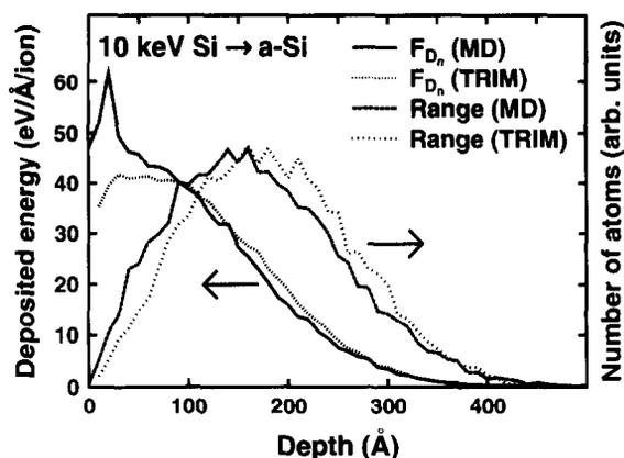
Fig. 6. Deposited energies and range profiles for implantation of 10 keV  $^{30}\text{Si}$  in a-Si calculated with the TRIM and MDRANGE programs.
