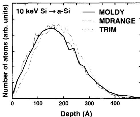
Fig. 3. MD and BCA range profiles of 10 keV Si implantation in a-Si.
