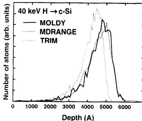
Fig. 4. MD and BCA range profiles of 40 keV H implantation in c-Si.
