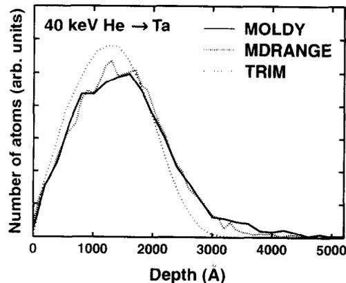
Fig. 5. MD and BCA range profiles of 40 keV He implantation in Ta.
