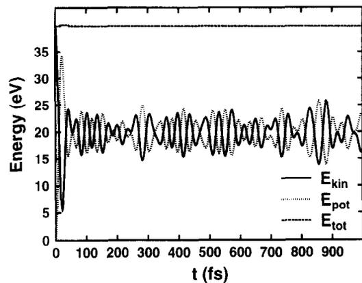
Fig. 1. Conservation of energy during an initial displacement calculation in the MDRANGE program.
