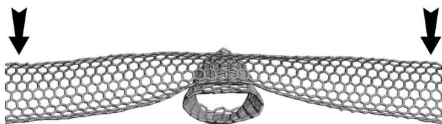
FIG. 6. Cross section along the axis of one of the crossed pristine nanotubes when a force of about 30 nN pushes one nanotube to the other. Although the force resulted in a substantial decrease of the intertube separation and mechanical deformation of the carbon network, welding of nanotubes does not occur even at elevated temperatures up to 2000 K.
