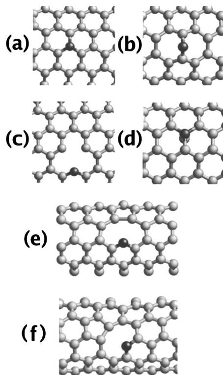
FIG. 1. Most abundant atomic configurations after B/N ion impacts onto single-walled carbon nanotubes. (a) perfect  $sp^2$  impurity, (b) bridge, (c) rocket, and (d)  $sp^2+C$  configurations in a (10,10) SWNT as calculated with the analytical model. The dark spheres represent the dopant atom, the light ones carbon atoms. (e) and (f) The rocket configurations in a (5,5) SWNT as calculated with the DFT model. Note partial mending of the defects by dangling bond saturation.
