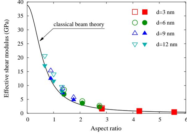
**Figure 7.** Dependence of the effective shear modulus on the aspect ratio of the nanorods. Open symbols indicate simulations in which all substrate atoms were fixed, while filled symbols correspond to simulations in which only the bottom layer of the substrate was fixed.
