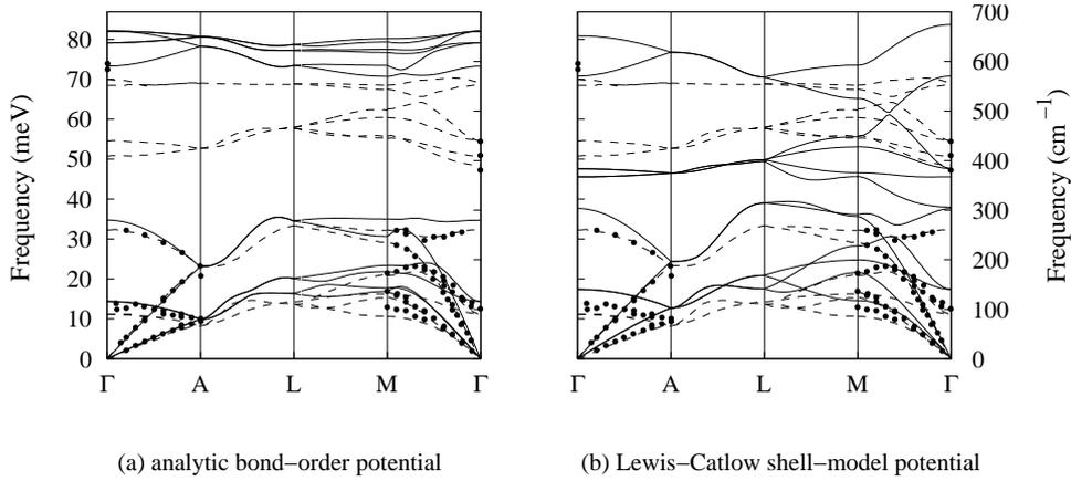
**Figure 3.** Phonon dispersion relations for (a) the analytic bond-order potential (—) developed in the present work and (b) the shell-model potential by Lewis and Catlow. Dashed lines (- - -) and black circles (●) show data from density-functional theory calculations and experiment, respectively [10].
