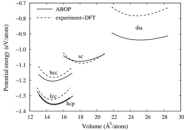
**Figure 4.** Energy-volume curves for bulk structures of zinc as obtained from the analytic bond-order potential (ABOP) in comparison with reference curves which were obtained by combining data from experiment and density-functional theory (DFT) calculations.
