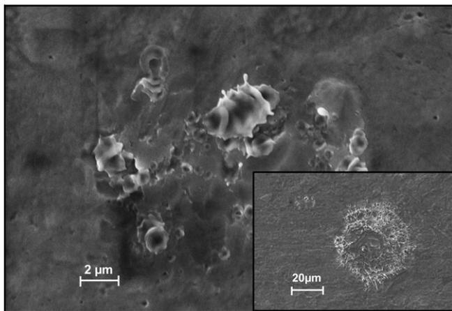
**Fig. 1.** Experimental craters on a Cu surface caused by the plasma formed in the high electric field ( $E_0 \approx 400 \frac{\text{MeV}}{\text{m}}$ ). The inset in the right bottom corner shows the overall view of the entire damaged area.
