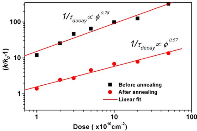
**Figure 4.** The dependence of the relative relaxation rate ( $k/k_0 - 1$ ) on the ion dose ( $\phi$ ). The solid lines are linear fit. The slope ( $\alpha$ ) for irradiated samples is  $0.78 \pm 0.06$  and for the irradiated-annealed sample is  $0.57 \pm 0.04$ . Since  $k/k_0 \gg 1$  in the entire dose regime, therefore  $k = 1/\tau_{\text{decay}} \propto \phi^\alpha$ .
