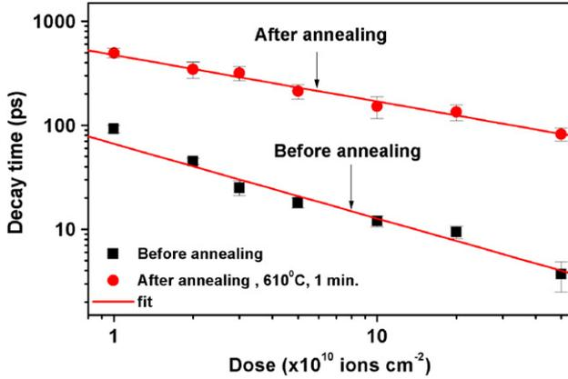
**Figure 2.** The decay times of irradiated and subsequently annealed GaInAs/InP QWs as a function of irradiation dose.
