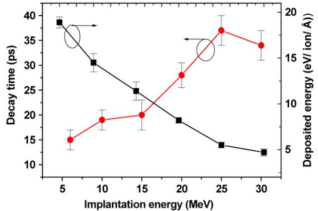
**Figure 5.** The decay time (●) and deposited energy (■) in the active region of GaInAs/InP QWs structure irradiated at  $5 \times 10^{10}$  ions  $\text{cm}^{-2}$   $\text{Ni}^+$  dose, as a function of implantation energy.
