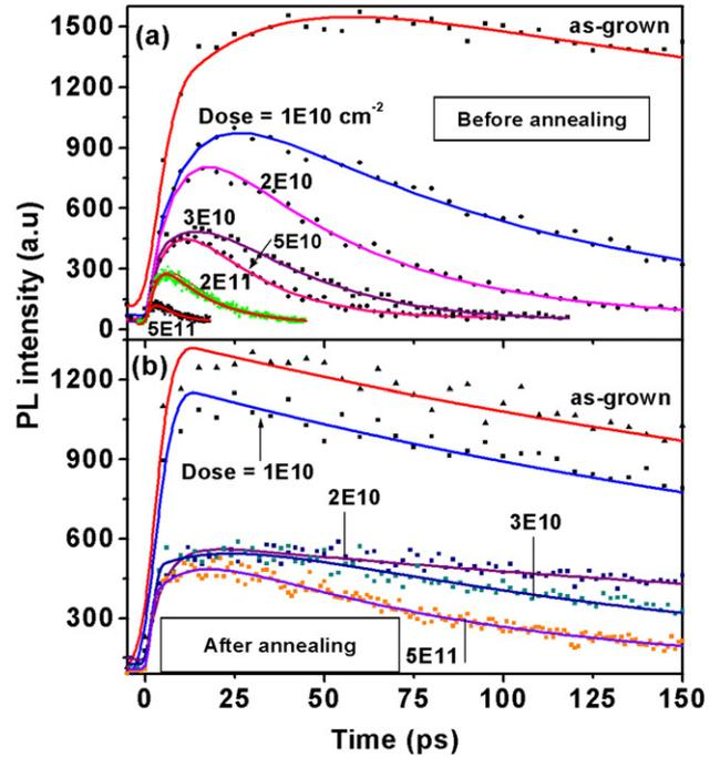
**Figure 1.** The time evolution of PL after the photo-excitation of GaInAs/InP QWs at different 10 MeV Ni<sup>+</sup> doses: (a) before annealing and (b) after annealing at 610 °C for 60 s.
