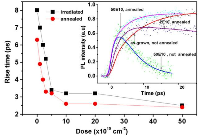
**Figure 3.** The PL rise time ( $\approx$  carrier capture time) for irradiated and annealed samples as a function of irradiation dose. The inset highlights the experimental PL profiles for a few selected samples.
