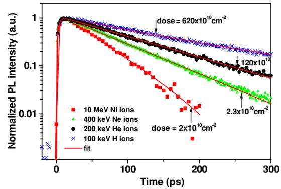
**Figure 1.** Selective TRPL decay profiles of InGaAs/GaAs QWs irradiated with  $\text{Ni}^+$ ,  $\text{Ne}^+$ ,  $\text{He}^+$  and  $\text{H}^+$  ions at different doses.
