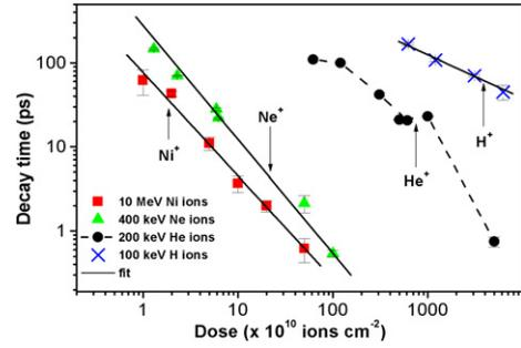
**Figure 4.** Decay time as a function of irradiation dose for different light and heavy ions. The desired decay time decrease is obtained with all the ions, but for  $\text{Ni}^+$  and  $\text{Ne}^+$  a much lower number of incident ions are needed to create the same decay time effect than for  $\text{H}^+$  and  $\text{He}^+$ .
