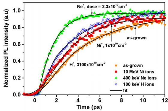
**Figure 2.** Time evolution (rise) of the PL signal from the as-grown sample ( $\tau_{\text{dec.}} = 455 \text{ ps}$ ) and the samples irradiated by different ions, but each with the same lifetimes of about 70 ps. The PL rise profile corresponding to  $\text{He}^+$  was similar to that of  $\text{H}^+$  and is not shown here for clarity. Among the different ions with similar decay times, the fastest capture dynamics can be seen for the  $\text{Ne}^+$  ion.
