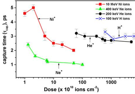
**Figure 3.** Carrier capture time ( $\tau_{\text{cap}}$ ) for different light and heavy ions as a function of irradiation dose. The capture time (not shown here) for the as-grown sample was 6 ps. The carrier capture time is almost independent of the dose for the light ions  $\text{He}^+$  and  $\text{H}^+$ .
