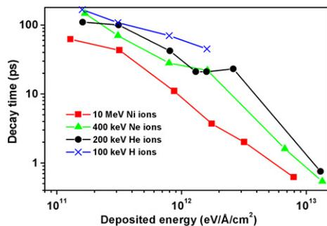
**Figure 5.** Decay time as a function of deposited energy for different light and heavy ions. The implantation energy for each ion is chosen such that similar penetration depth and deposited energy profiles are obtained. The nuclear deposited energies per ion are 1.2, 60 and 620 times smaller for  $\text{Ne}^+$ ,  $\text{He}^+$  and  $\text{H}^+$  compared to  $\text{Ni}^+$ .
