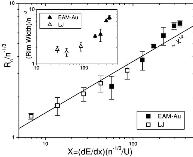
FIG. 6. Crater dimensions versus scaled  $dE/dx$  for both EAM Au and a LJ solid. The LJ results are from Ref. 52.  $dE/dx$  was obtained from SRIM for the Au results.
