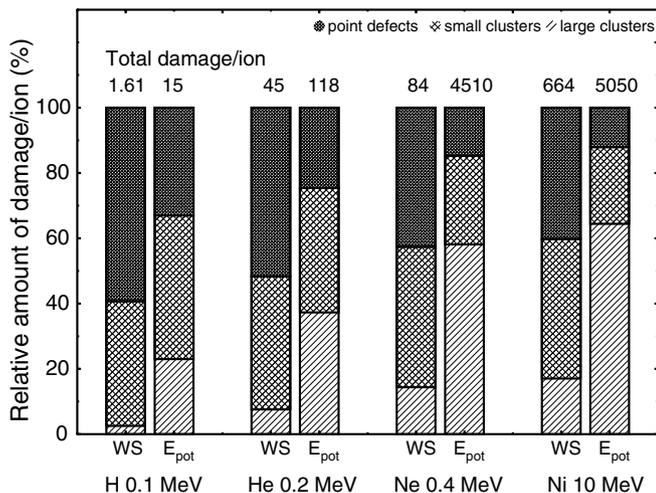
Fig. 3. The final defect distribution of the implantation. The total amount of damage per ion, as well as the fraction of defects in clusters of different sizes, is shown for both the Wigner–Seitz (WS) and the potential energy ( $E_{\text{pot}}$ ) analysis.
