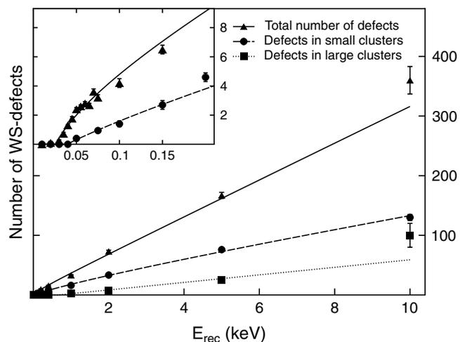
Fig. 1. The number of Wigner–Seitz-defects (WS-defects) (vacancies and interstitials) produced by collision cascades initiated by As-recoils in GaAs. Small clusters contain 2–10 WS-defects. The inset shows the defect production at low recoil energies.
