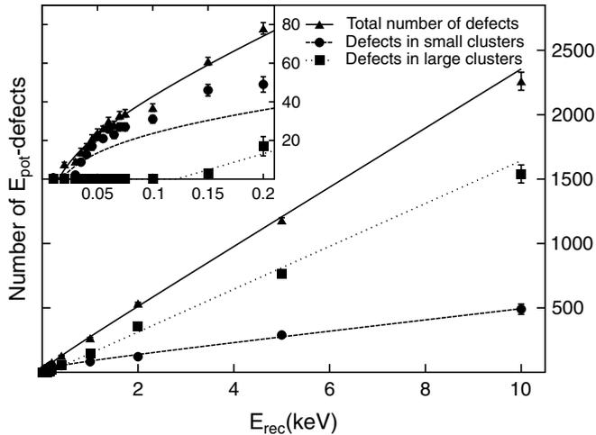
Fig. 2. The number of atoms with a potential energy of more than 0.2 eV above equilibrium value ( $E_{\text{pot}}\text{-defects}$ ) after collision cascades in GaAs. Small clusters are clusters containing 10–70 defects. The inset illustrates the amount produced at low recoil energies.
