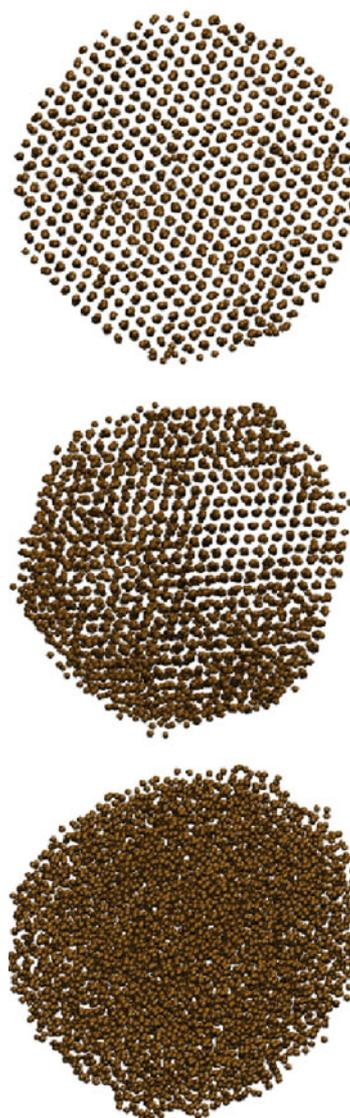
**Fig. 2.** A gold nanocluster of diameter 6 nm (a) before melting, (b) at the onset of melting, and (c) after melting. Note the transition from spherical cluster in (a) to faceted at elevated temperatures in (b).
