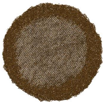
**Fig. 1.** Cross-section of an 18 nm nanocluster melting from the surface inward.
